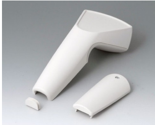
A9056107 SENSO-CASE M ABS (UL 94 HB) off-white RAL 9002 7.09"x3.39"x1.77" IP 41
