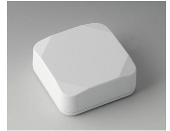
B1804217 MINI-DATA-BOX S50, high ASA+PC (UL 94 V-0) traffic white RAL 9016 1.97"x1.97"x0.79" IP 65 opt., IP 40
