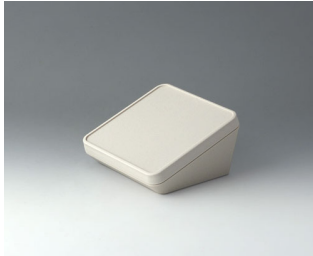
B4414107 PROTEC 140, Vers. I ASA+PC-FR (UL 94 V-0) off-white RAL 9002 5.51"x5.51"x2.99" IP 65 opt.
