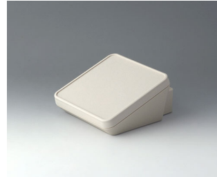
B4414307 PROTEC 140, Vers. III ASA+PC-FR (UL 94 V-0) off-white RAL 9002 5.51"x6.30"x2.99" IP 65 opt.
