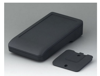
A9006218 DATEC-COMPACT M ASA+PC (UL 94 V-0) lava 6.77"x3.62"x1.54" IP 41
