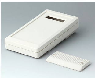
A9073307 DATEC-MOBIL-BOX S, Vers. III ABS (UL 94 HB) off-white RAL 9002 5.98"x3.27"x1.32" IP 65 opt.
