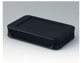
A9052209 SOFT-CASE L PMMA (IR) (UL 94 HB) black RAL 9005 2.87"x4.61"x0.94" IP 54 opt., IP 40
