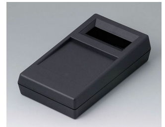
A9061119 HAND-HELD-BOX N, Vers. II ABS (UL 94 HB) black RAL 9005 7.09"x3.94"x1.73"
