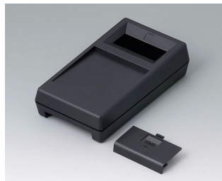
A9062019 HAND-HELD-BOX M, Vers. I ABS (UL 94 HB) black RAL 9005 5.71"x3.15"x1.52"
