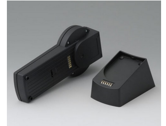
A9076159 SET: DATEC-CONTROL XS, Vers. I, station.. ABS (UL 94 HB) black RAL 9005 7.87"x3.70" IP 65 opt.
