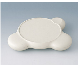
B2514107 BLOB PANEL ABS (UL 94 HB) off-white RAL 9002 7.87"x6.50"x1.42" IP 54 opt.
