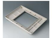
B4046717 Bottom part L flat, version II ABS (UL 94 HB) off-white RAL 9002 10.83"x7.68"x1.04" IP 54 opt.
