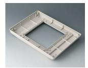
B4044707 Bottom part M flat, version I ABS (UL 94 HB) off-white RAL 9002 8.86"x6.50"x1.00" IP 54 opt.
