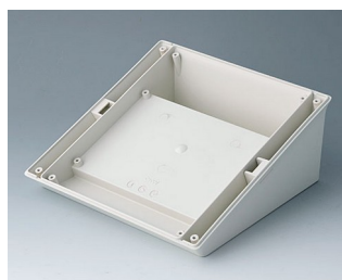
B4046827 Base L - desk-top - ABS (UL 94 HB) off-white RAL 9002 7.20"x7.20"x2.87"
