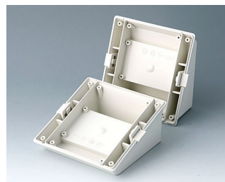
B4042847 Base S - desk-top/wall - ABS (UL 94 HB) off-white RAL 9002 4.84"x4.84"x2.09"
