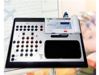
Stationary system for long-term EEG recordings
