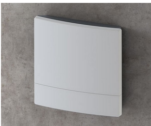
B3222101 NET-BOX 220, Vers. I ASA+PC (UL 94 V-0) light gray RAL 7035 8.66"x8.66"x1.99" IP 65 opt., IP 40
