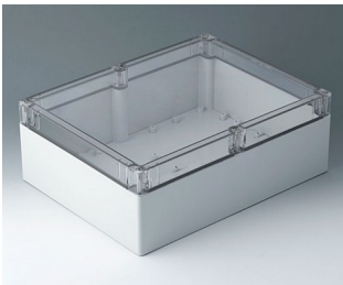
C7030114 IN-BOX ABS/PC (UL 94 HB) light gray RAL 7035 11.89"x9.13"x4.33" IP 66, IP 67, IK 07
