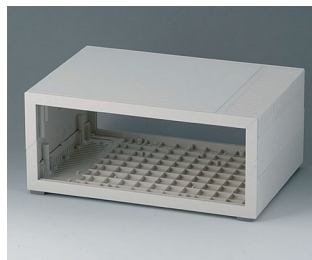
B2211207 MEDITEC D 160, without handle bar ABS (UL 94 HB) off-white RAL 9002 11.42"x7.87"x4.88" IP 40
