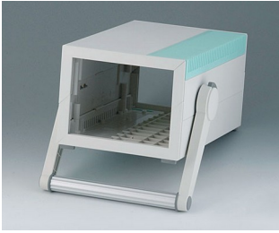
B2212305 MEDITEC E 220, with handle bar ABS (UL 94 HB) off-white RAL 9002 6.30"x10.24"x4.88" IP 40
