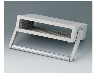
B2211107 MEDITEC D 160, with handle bar ABS (UL 94 HB) off-white RAL 9002 11.42"x7.87"x2.91" IP 40
