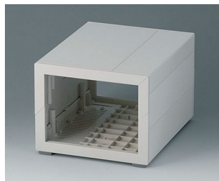
B2213217 MEDITEC E 160, without handle bar ABS (UL 94 HB) off-white RAL 9002 6.30"x7.87"x4.88" IP 40
