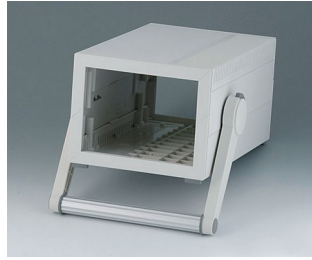
B2212307 MEDITEC E 220, with handle bar ABS (UL 94 HB) off-white RAL 9002 6.30"x10.24"x4.88" IP 40
