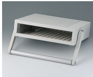
B2210107 MEDITEC D 220, with handle bar ABS (UL 94 HB) off-white RAL 9002 11.42"x10.24"x2.91" IP 40
