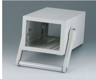
B2212317 MEDITEC E 220, with handle bar ABS (UL 94 HB) off-white RAL 9002 6.30"x10.24"x4.88" IP 40
