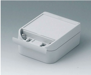
C6009121 SMART-BOX WIDTH 3.543" ASA+PC (UL 94 V-0) light gray RAL 7035 4.72"x3.54"x1.97" IP 66
