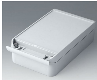
C6013221 SMART-BOX WIDTH 5.118" ASA+PC (UL 94 V-0) light gray RAL 7035 8.66"x5.12"x2.36" IP 66
