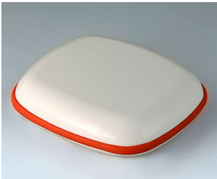
B1608107 BODY-CASE XL, without recess ASA (UL 94 HB) traffic white RAL 9016 2.44"x2.20"x0.71" IP 65
