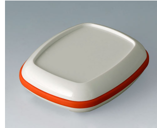
B1604207 BODY-CASE M, with recess ASA (UL 94 HB) traffic white RAL 9016 1.97"x1.61"x0.63" IP 65
