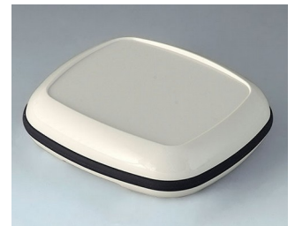
B1608217 BODY-CASE XL, with recess ASA (UL 94 HB) traffic white RAL 9016 2.44"x2.20"x0.67" IP 65
