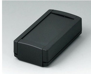
B1040369 TOPTEC 102, Vers. I ABS (UL 94 HB) black RAL 9005 4.02"x2.13"x1.18" IP 40
