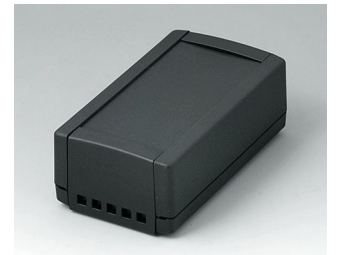
B1050469 TOPTEC 123 H, Vers. II ABS (UL 94 HB) black RAL 9005 4.84"x2.68"x1.77" IP 40
