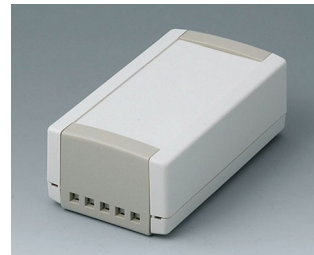
B1050465 TOPTEC 123 H, Vers. II ABS (UL 94 HB) off-white RAL 9002 4.84"x2.68"x1.77" IP 40
