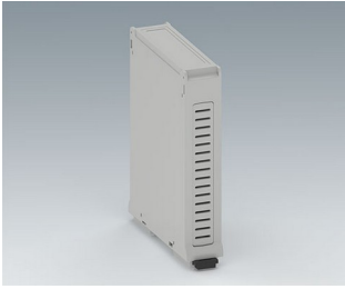
B6522103 RAILTEC BP, M22, with ventilation slots PC (UL 94 V-0) light gray RAL 7035 3.74"x0.91"x4.45"
