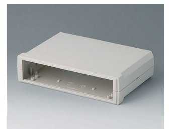
B3020117 MOTEC M, flat/flat ABS (UL 94 HB) off-white RAL 9002 8.07"x5.51"x1.97" IP 40
