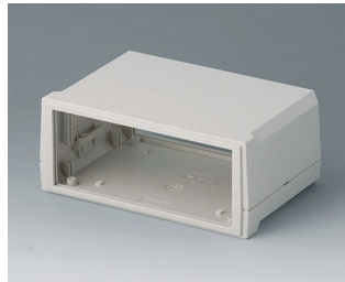
B3015127 MOTEC S, flat/high ABS (UL 94 HB) off-white RAL 9002 6.10"x4.13"x2.56" IP 40
