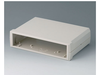
B3023117 MOTEC-L, flat/flat ABS (UL 94 HB) off-white RAL 9002 9.25"x6.50"x2.36" IP 40
