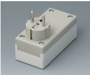
A9011665 PLUG CASE F / D, Vers. I PC+ABS (UL 94 V-0) off-white RAL 9002 3.94"x1.97"x1.57"
