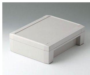
C8017222 SOLID-BOX 175 PC+ABS (UL 94 V-0) light gray RAL 7035 8.86"x6.89"x2.76" IP 66, IP 67, IK 08
