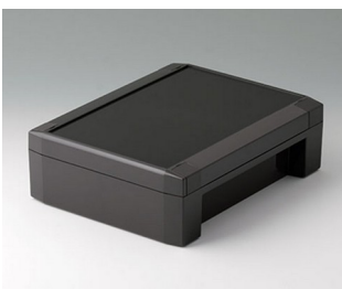
C8017221 SOLID-BOX 175 PC+ABS (UL 94 V-0) anthracite gray RAL 7016 8.86"x6.89"x2.76" IP 66, IP 67, IK 08
