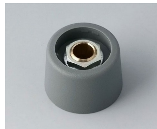
A3123638 COM-KNOBS 23, without recess PA 6 volcano 23x16mm 1/4"
