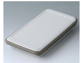
B5403217 SLIM-CASE M, Vers. V ASA+PC-FR (UL 94 V-0) off-white RAL 9002 5.83"x2.91"x0.87" IP 54
