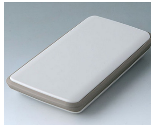
B5403117 SLIM-CASE M, Vers. IV ASA+PC (UL 94 V-0) off-white RAL 9002 5.83"x2.91"x0.87" IP 54
