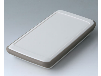
B5403217 SLIM-CASE M, Vers. V ASA+PC-FR (UL 94 V-0) off-white RAL 9002 5.83"x2.91"x0.87" IP 54
