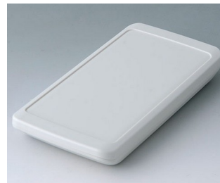
B5403207 SLIM-CASE M, Vers. II ASA+PC (UL 94 V-0) off-white RAL 9002 5.83"x2.91"x0.75" IP 65 opt., IP 40
