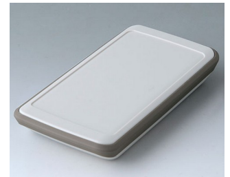
B5403217 SLIM-CASE M, Vers. V ASA+PC (UL 94 V-0) off-white RAL 9002 5.83"x2.91"x0.87" IP 54
