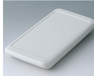
B5403207 SLIM-CASE M, Vers. II ASA+PC-FR (UL 94 V-0) off-white RAL 9002 5.83"x2.91"x0.75" IP 65 opt., IP 40
