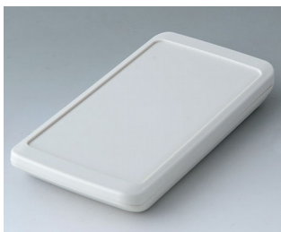
B5403307 SLIM-CASE M, Vers. III ASA+PC-FR (UL 94 V-0) off-white RAL 9002 5.83"x2.91"x0.75" IP 65 opt., IP 40
