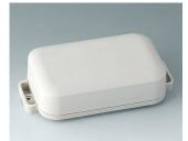
C3207207 EASYTEC 125 ASA+PC (UL 94 V-0) off-white RAL 9002 5.79"x3.07"x1.46" IP 65 opt., IP 40
