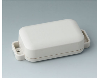
C3204207 EASYTEC 80 ASA+PC-FR (UL 94 V-0) off-white RAL 9002 3.98"x1.97"x1.02" IP 65 opt., IP 40
