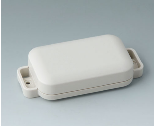
C3204107 EASYTEC 80 ASA+PC-FR (UL 94 V-0) off-white RAL 9002 3.98"x1.97"x0.87" IP 65 opt., IP 40
