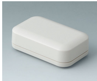
A9403107 EVOTEC 80, Vers. I ASA+PC-FR (UL 94 V-0) off-white RAL 9002 3.15"x1.97"x1.02" IP 65 opt., IP 40
