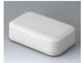
A9443107 EVOTEC 150, Vers. I ASA+PC-FR (UL 94 V-0) off-white RAL 9002 5.91"x3.66"x1.77" IP 65 opt., IP 40
