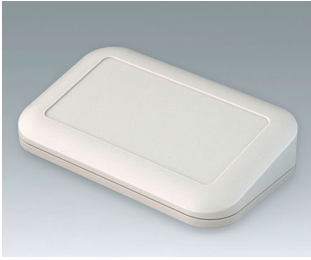
A9446107 EVOTEC 150, Vers. III ASA+PC-FR (UL 94 V-0) off-white RAL 9002 5.91"x3.66"x1.42" IP 65 opt., IP 40
