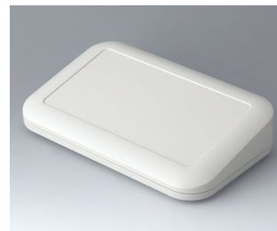
A9466107 EVOTEC 200, Vers. III ASA+PC-FR (UL 94 V-0) off-white RAL 9002 7.87"x4.88"x1.77" IP 65 opt., IP 40
