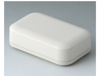
A9423107 EVOTEC 100, Vers. I ASA+PC-FR (UL 94 V-0) off-white RAL 9002 3.94"x2.44"x1.22" IP 65 opt., IP 40
