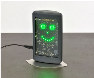
Room air measuring device
