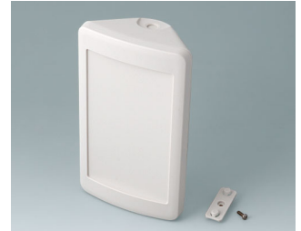
B4610207 SMART-CONTROL M, Vers. II ASA+PC-FR (UL 94 V-0) off-white RAL 9002 6.81"x3.98"x2.32" IP 55 opt., IP 40
