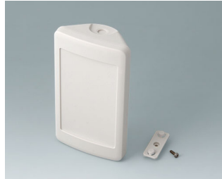
B4608207 SMART-CONTROL S, Vers. II ASA+PC-FR (UL 94 V-0) off-white RAL 9002 5.59"x3.19"x1.81" IP 55 opt., IP 40
