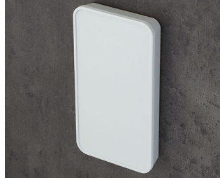
C6406107 SMART-PANEL E155 ASA+PC-FR (UL 94 V-0) traffic white RAL 9016 6.10"x3.31"x0.84" IP 40
