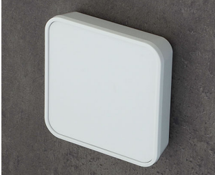
C6402107 SMART-PANEL S84 ASA+PC-FR (UL 94 V-0) traffic white RAL 9016 3.31"x3.31"x0.84" IP 40
