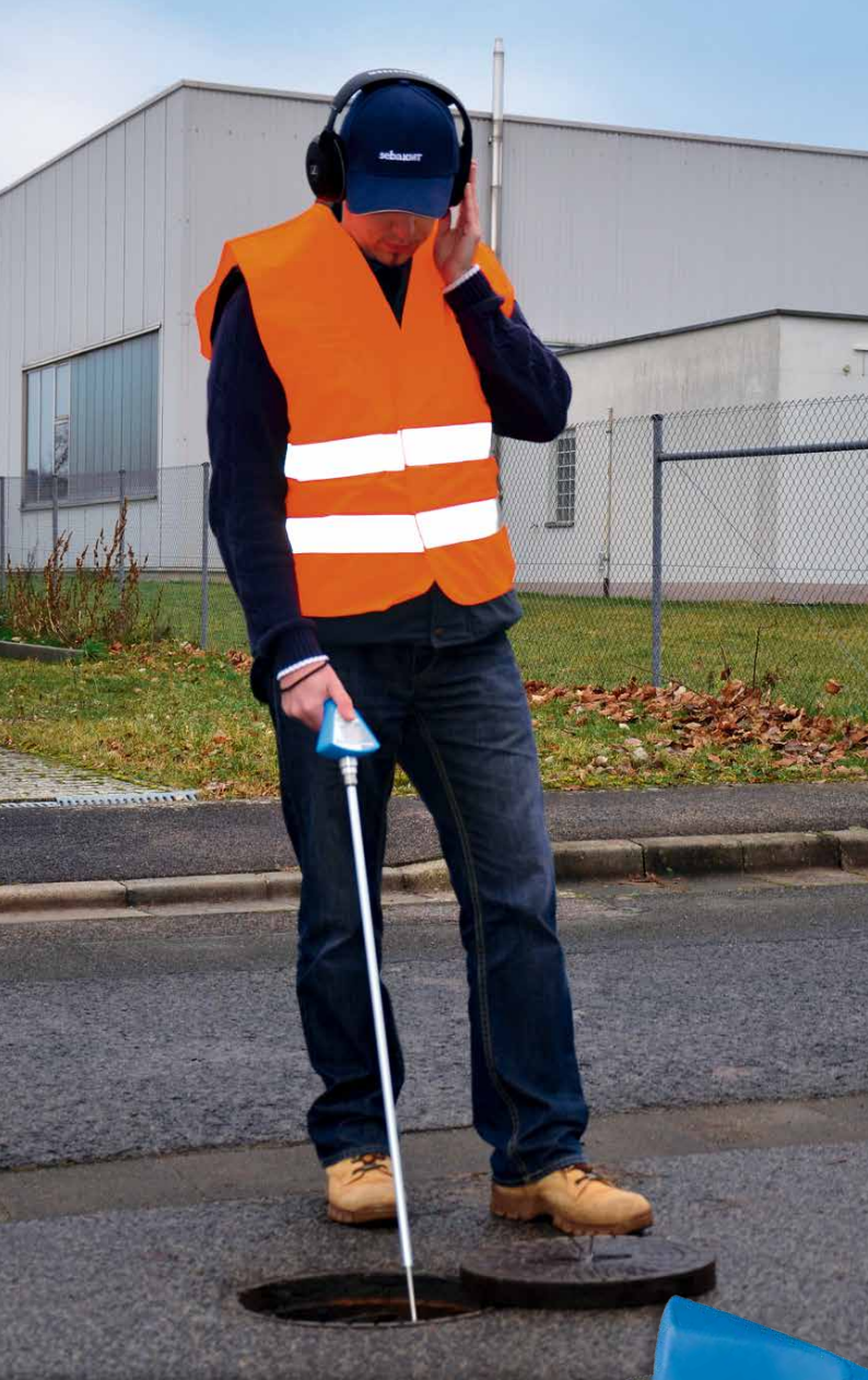
HYDROLUX HL 50 – Portable leak detection unit with integrated sensor and cordless headsets.
