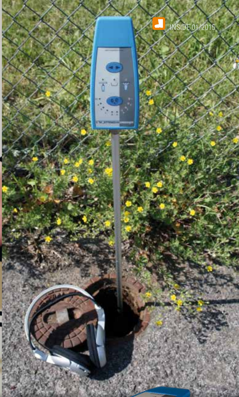
HYDROLUX HL 5 – The mini water leak detection unit with visual and audible leak display (OKW mobile enclosure series SMART-CASE).
